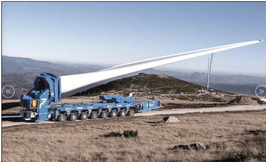
Figure 2: Specialist blade lifting unit.
